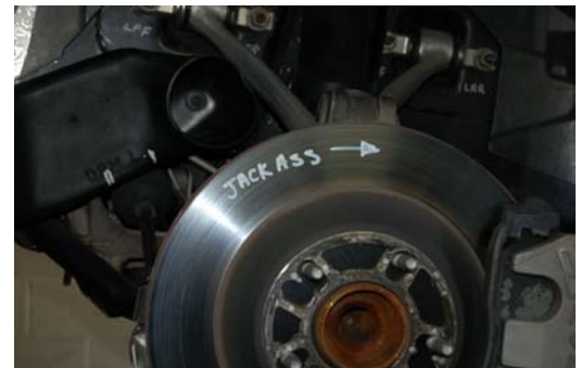
A message left on the 10/10ths Race Car when it was found to have the front rotors on backwards.
