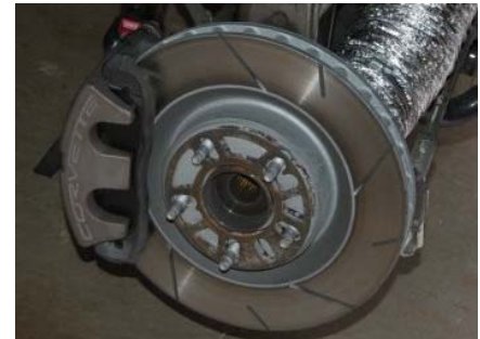
Slotted rotors with slanted vanes.
